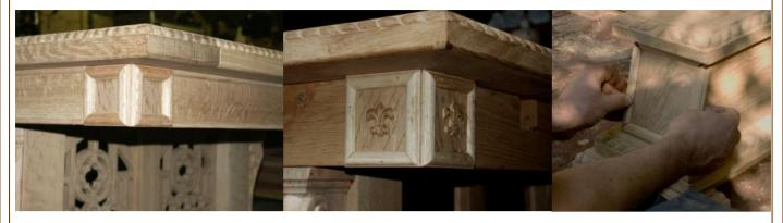
All surfaces that are end grain on exposed faces are covered using an 1/8" thick face plate. Moldings are placed around the corner blocks, feet faces, and aprons, as well as framing the panels. Use of appliqués is very common to provide subtle ornate features to the piece.
