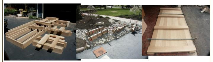
Planks are cut from our predetermined cut-sheets, then blanks are glued up to form the leg structures and pieces requiring lamination of multiple 8/4 layers to reach their final thickness. Everything is proportionate to the table surface, so the surfaces are laid out first in rough form, then the formal joint work begins.
