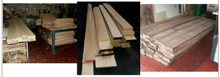
Creating a New Wave Gothic piece starts out with a rather large pile of wood; the average dining table requiring over 1000lbs of rough lumber. After a significant amount of rips, cross cuts, planing, jointing, sanding, drilling, scraping, sawing, and carving the net weight is around 500lbs.
